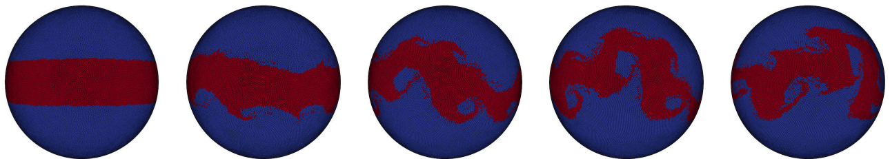
Figure 5: Particle-based simulation of an incompressible fluid on a rotating sphere using the Gallouët-Mérigot scheme [1]. The complete simulation can be viewed here.
