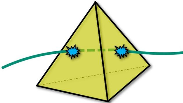
Figure 2: CAD-Curve to Overlay-Tri Intersection
