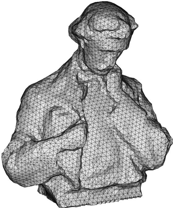
Figure 5: Edgar Allan Poe size 3.0, 103,170 tetrahedral elements, 14 MPI procs, 26 seconds generation time, min scaled Jacobian: 0.113
