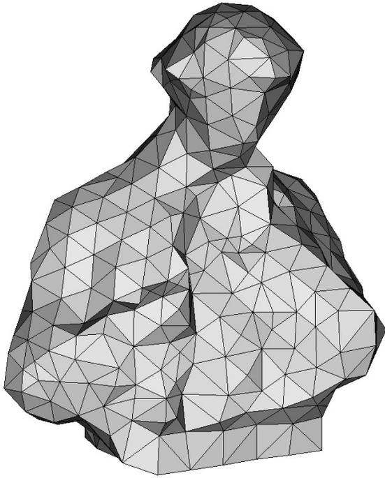
Figure 4: Edgar Allan Poe size 10.0, 2,882 tetrahedral elements, 14 MPI procs, 14 seconds generation time, min scaled Jacobian: 0.226
