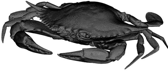
Figure 8: The IMR crab, 7.6M tetrahedral elements, 14 MPI procs, 531 seconds generation time, min scaled Jacobian: 0.126
