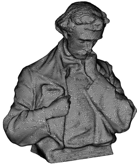
Figure 6: Edgar Allan Poe size 1.0, 2.78M tetrahedral elements, 14 MPI procs, 74 seconds generation time, min scaled Jacobian: 0.129
