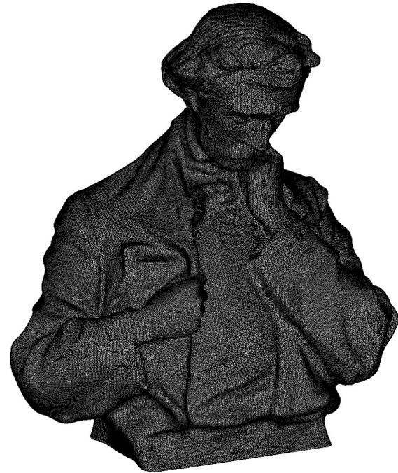
Figure 7: Edgar Allan Poe size 0.5, 22.2M tetrahedral elements, 14 MPI procs, 392 seconds generation time, min scaled Jacobian: 0.135
