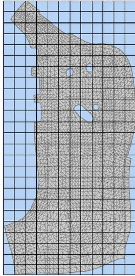
Figure 2: A possible Beziér mesh for fitting a 1996 Dodge Neon A-pillar component [5] is shown, as would be defined by knot vectors in the  $u$ - and  $v$ -directions.
