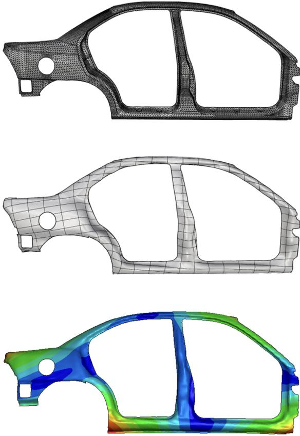
Figure 4: A Dodge Neon cabin side panel mesh [5], rebuilt geometry, and modal analysis are shown.
