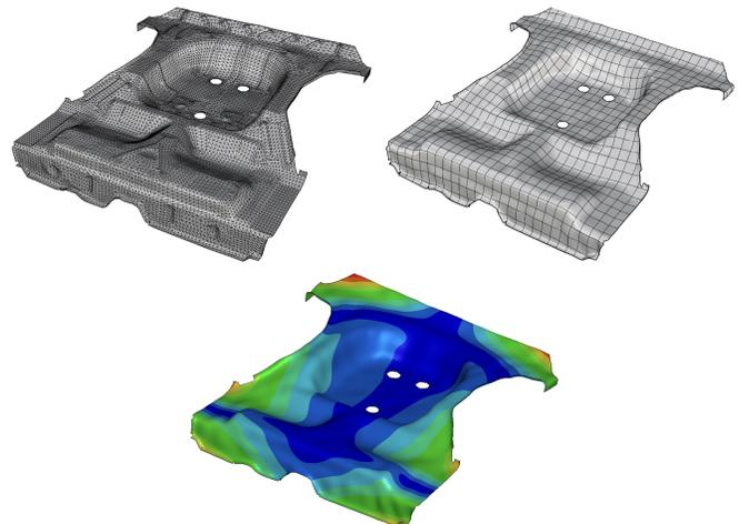
Figure 3: A Dodge Neon floorboard mesh [5], rebuilt geometry, and modal analysis are shown.
