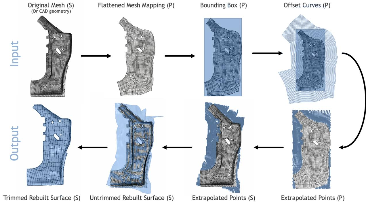
Figure 1: The process by which a single trimmed surface is created from an original CAD geometry (or its mesh) is displayed. Spatial and parametric domains are denoted by (S) and (P), respectively. The geometry of interest for this graphic is a component of a 1996 Dodge Neon A-pillar [5], whose biquadratic reconstruction is made using 484 control points.
