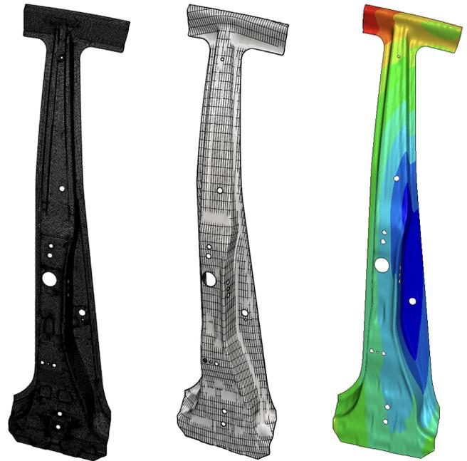
Figure 5: A Honda B-pillar geometry [14], rebuilt geometry, and modal analysis are shown.
