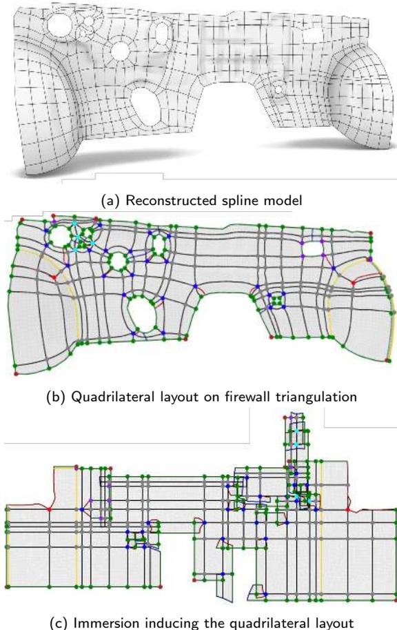
**Figure 1:** Above, the firewall of a 1996 Dodge Neon is rebuilt as a union of B-spline patches that are defined based on a quadrilateral layout computed and defined on the triangulation in the center. This quadrilateral layout is induced by the immersion map below, and is the result of Ricci flow with metric optimization.
