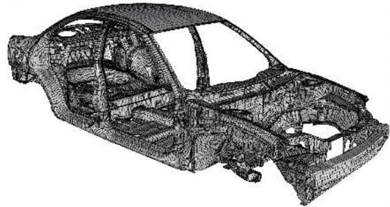
**Figure 2:** Reconstructed isogeometric model of the George Washington University 1996 Dodge Neon body-in-white finite element model [9].
