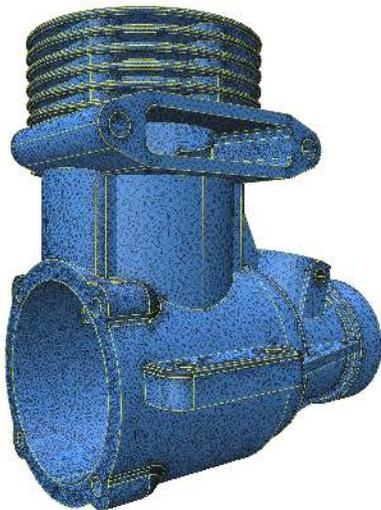
**Figure 1:** Remesh result for the Crank model.
