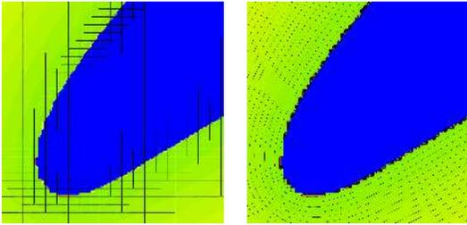
Figure 4: Zoom at the left tip of the blade showing the oscillating cut elements around the zero level set of  $\sigma_{0B}$ .
