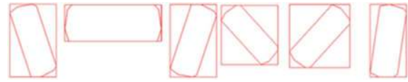
Fig. 6. A set of 2D oriented bounding boxes for different orientations of convex hull
