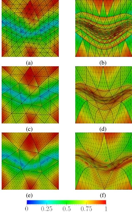
**Figure 6:** Point-wise distortion for triangular meshes of polynomial degree 1, 2 and 4 in rows. Initial straight-sided isotropic meshes and optimized meshes from initial meshes in columns. The interpolation of the metric has been used for the distortion minimization. The sub-triangular elements are the visualization elements. These element vertices are not the high-order degrees of freedom.
