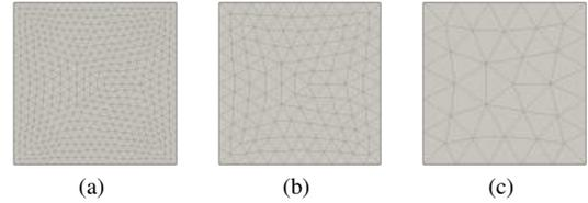
**Figure 5:** Background triangular meshes of polynomial degree 1, 2 and 4.
