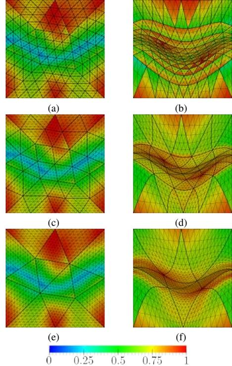
**Figure 7:** Point-wise distortion for triangular meshes of polynomial degree 1, 2 and 4 in rows. Initial straight-sided isotropic meshes and optimized meshes from initial meshes in columns. The analytic evaluation of the metric has been used for the distortion minimization.
