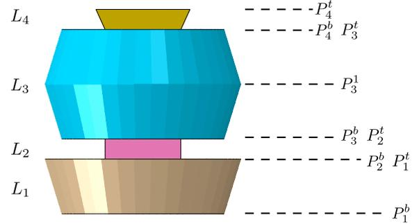
(a)  $L_1$  and  $L_4$  are defined by a pair of topologically equivalent polygon sets  $\{P_1^b, P_1^t\}$  and  $\{P_4^b, P_4^t\}$  respectively;  $L_3$  is defined by  $\{P_3^b, P_3^1, P_3^t\}$  where  $P_3^1$  is an intermediate polygon set;  $L_2$  is a straight layer defined by one polygon set, i.e.,  $P_2^b \equiv P_2^t$ . Note that  $\{P_3^b, P_2^b, P_1^t\}$  are in the same level as arranged in Table 1 as  $L_2$  is a straight layer.
