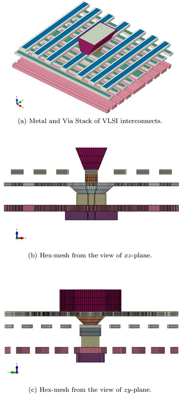
**Figure 2:** A VLSI Metal and Via Model composed of 8 layers.
