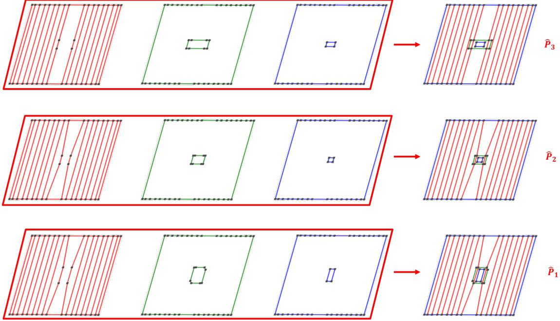
**Figure 8:** Merge all polygon sets at the same row into  $\mathcal{P} = \{\hat{P}_1, \hat{P}_2, \hat{P}_3\}$ ; Under the constraints of  $\hat{P}_1$ , a Delaunay triangulation is generated. As the merged polygon sets are topologically equivalent, a topologically equivalent triangulation of the other rows are generated accordingly. The triangulations form a multiple-layered map  $\Phi$ .
