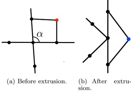
**Figure 10:**  $\alpha$  is a corner of polygon constraints of quadrilateral meshing. The red node on the left is extruded to the blue node on the right. The angle of  $\alpha$  is distorted to  $180^\circ$  after extrusion. In this case, the straightened edges are on the boundary of distinguished materials on the extruded layer. The invalid corner is unable to be fixed through optimizations.
