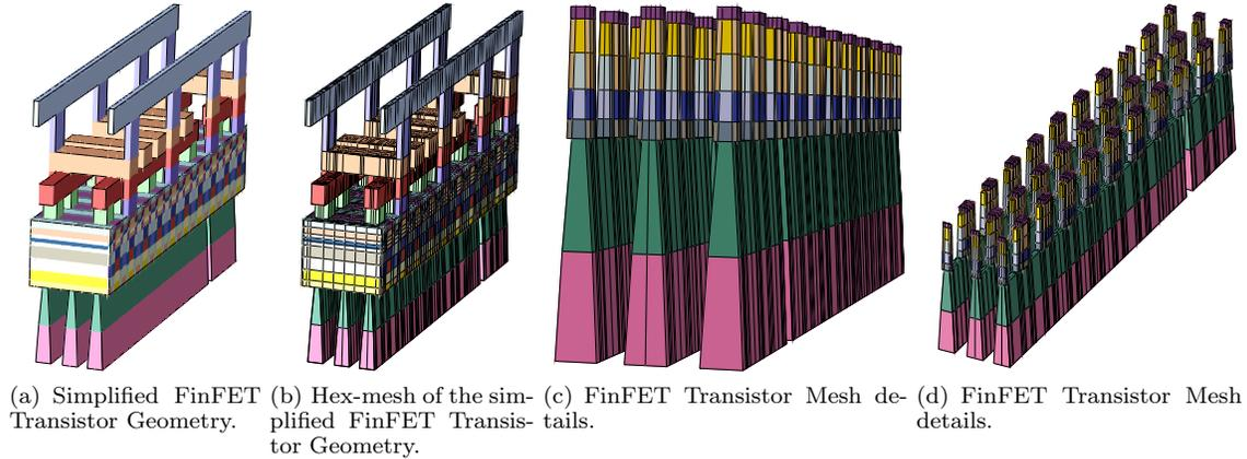
**Figure 1:** A Simplified FinFET transistor and metal interconnect model composed of 16 layers for Thermal Modeling. The generic name "FinFET" is given as the source/drain region forms fin-shaped bodies on the silicon surface.
