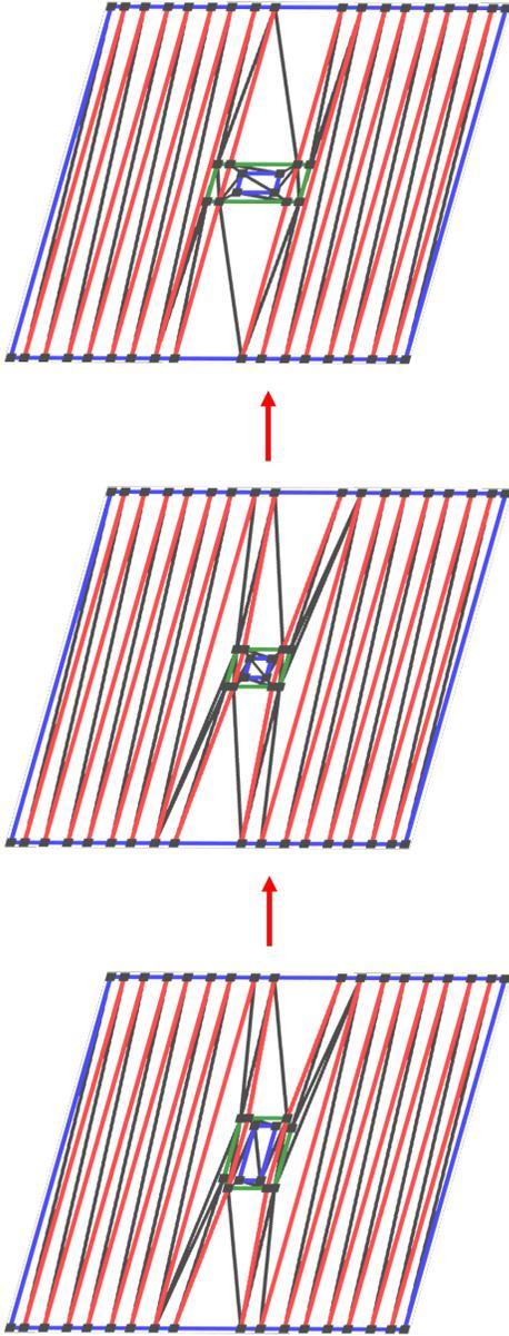
**Figure 9:** Generate a Delaunay triangulation under the constraint of the bottom polygon set. The number of polygons in the three sets is equal and the polygons are matched across the sets. That is, each polygon in a set is paired with one polygon in each of the other sets. Therefore, by referring to the triangulation at the bottom level, a triangulation with the same structure is constructed to each of the upper polygon sets.
