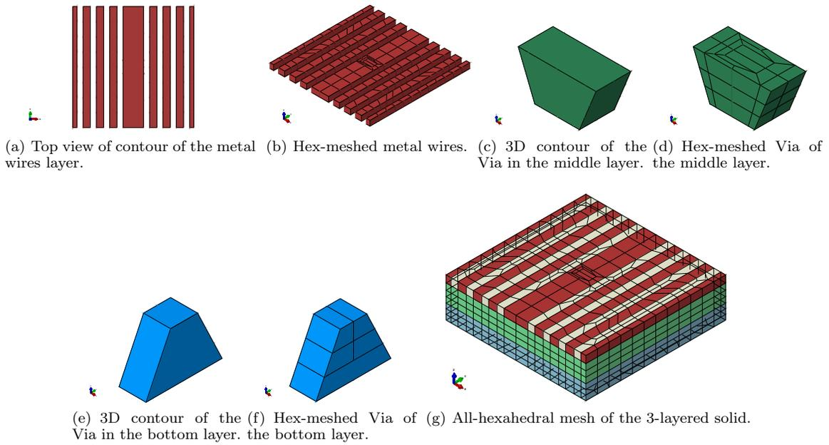
**Figure 3:** Hexahedral mesh of a model with three layers. The geometries of the layers are defined in a rectangle domain. The quad mesh is generated within the rectangular boundary and the hex-mesh is extruded along  $+z$ -axis. Aside from the metal wires and Vias, the other meshed volumes represent empty spaces whose materials are defined by air.
