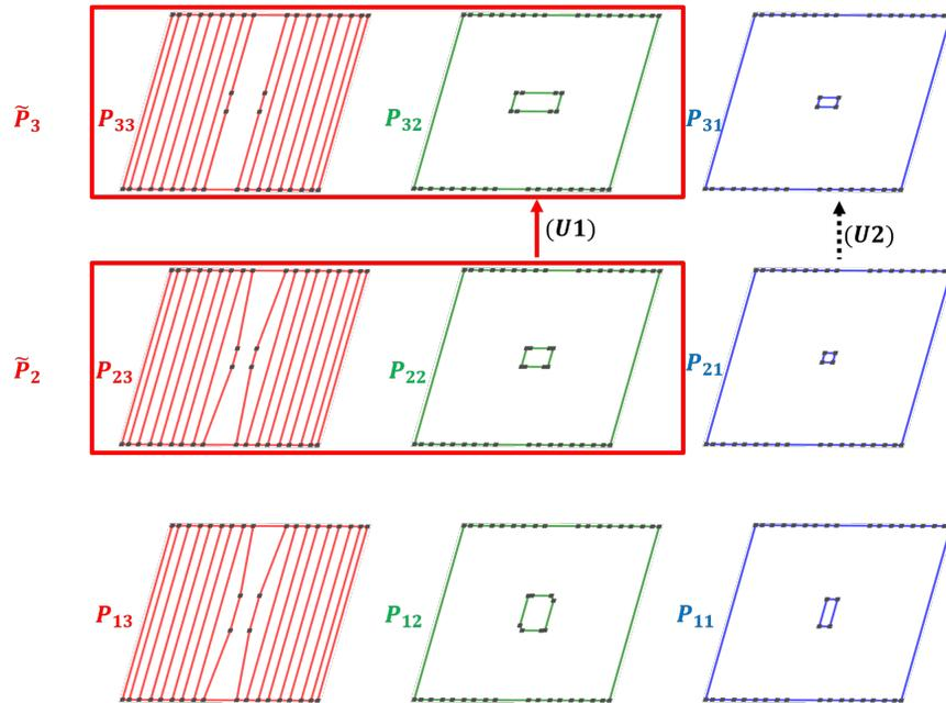
**Figure 7:** Polygon sets generation by upward mappings. (U1) Merge the polygon sets  $\{P_{23}, P_{22}\}$  of row 2 and  $\{P_{33}, P_{32}\}$  of row 3, and construct a map; (U2) Map  $P_{21}$  upward through the map.
