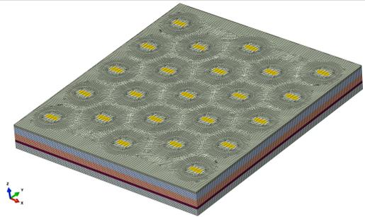
(c) All-hexahedral mesh of the 4-layered solid. All of the geometries are enclosed by a 2D rectangle domain.
