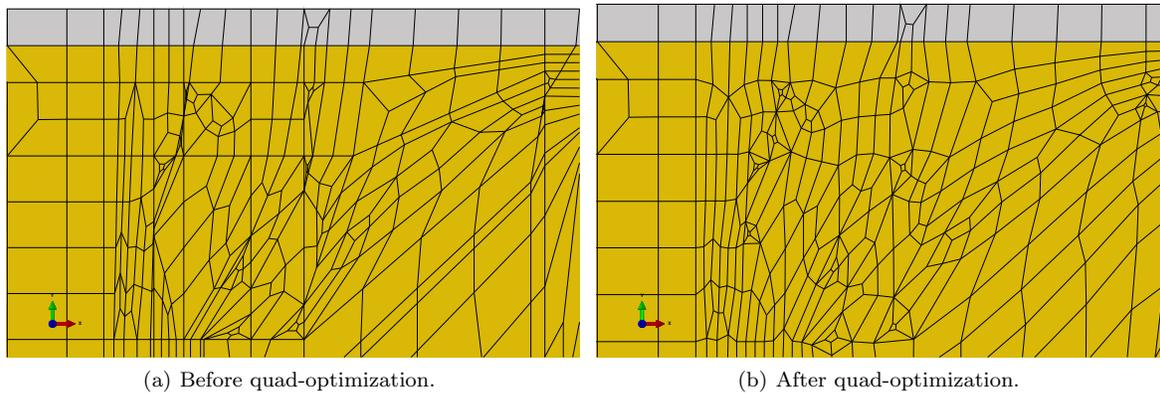
**Figure 11:** The snapshots show a comparison of mesh quality before and after quad-mesh optimization. The grey and yellow regions represent metal wires in some layer of the metal-Via model from the experimental results.
