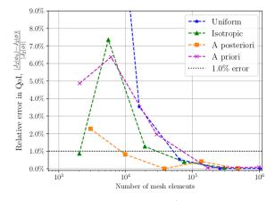
**Figure 7**: Relative error in  $J_2^{\text{exact}}$  and error estimator (16) evaluated on meshes arising from: uniform refinement; isotropic adaptation; a posteriori anisotropic adaptation; and a priori anisotropic adaptation.
