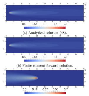
(c) Finite element adjoint solution corresponding to QoI  $J_1$  and receiver  $R_1$ .
