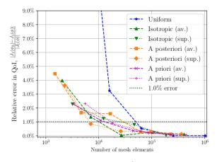
**Figure 5**: Relative error in  $J_1^{\text{exact}}$  resulting from mesh adaptation routines which combine forward and adjoint error metrics. Here *av.* and *sup*. denote 'average' and 'superposition', respectively.
