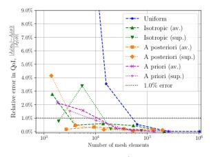
**Figure 9**: Relative error in  $J_2^{\text{exact}}$  resulting from mesh adaptation routines which combine forward and adjoint error metrics. Notation as in Figure 5.
