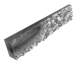
Figure 10: Clip of a mesh with 1,776,396 elements resulting from goal-oriented mesh adaptation for a 3D extension of the TELEMAC-2D test case discussed in Subsection 5.3. The metric is obtained by averaging forward and adjoint a posteriori anisotropic metrics.
