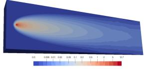
(b) Finite element solution on a 1,766,396 element mesh which was obtained by adaptation with respect to averaged forward and adjoint a posteriori metrics.
