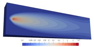
(a) Finite element solution on a uniform mesh with 1,920,000 elements.
