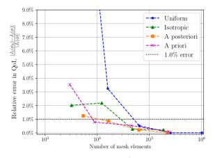
**Figure 3**: Relative error in  $J_1^{\text{exact}}$  for finite element solutions computed on meshes arising from: uniform refinement; isotropic adaptation; a posteriori anisotropic adaptation; and a priori anisotropic adaptation.
